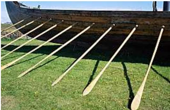
**These were the kind of oars used on Viking ships 900 years prior to the whaleboats. Made of pine they were lighter and the blades were better designed. The width of the blade is known from the slots cut in the side of salvaged wrecks to accommodate the blade. The beam and weight of these boats limited their rowing speed to 2-3 knots.**
