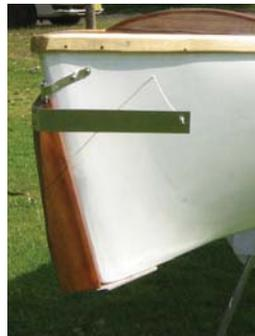
*Optional rudder in place controlled by the passenger in the stern seat.*
