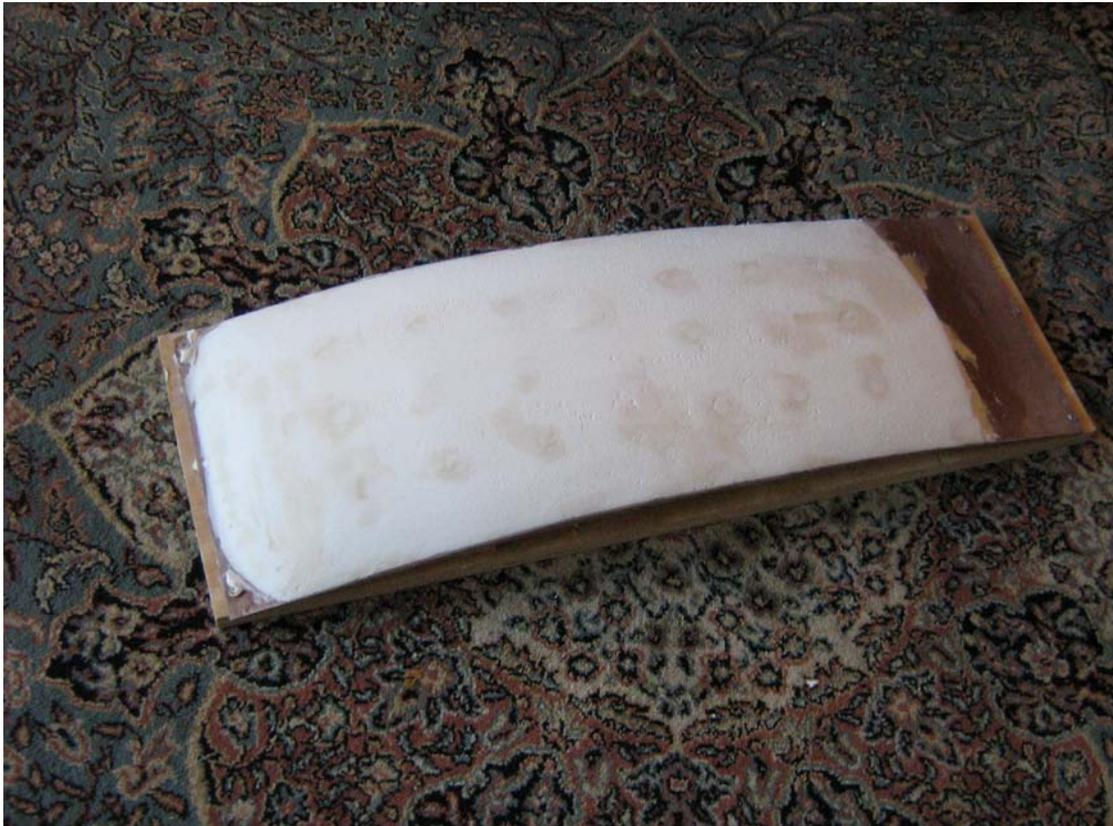
The Sailing blade mould before fibre glassing.
