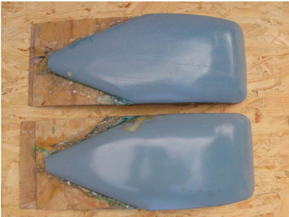
**The two asymmetric moulds for the Turbo blade. The curve at the bottom of each blade (outside of picture) is less severe to allow cleaner entry and exit from the water.**
