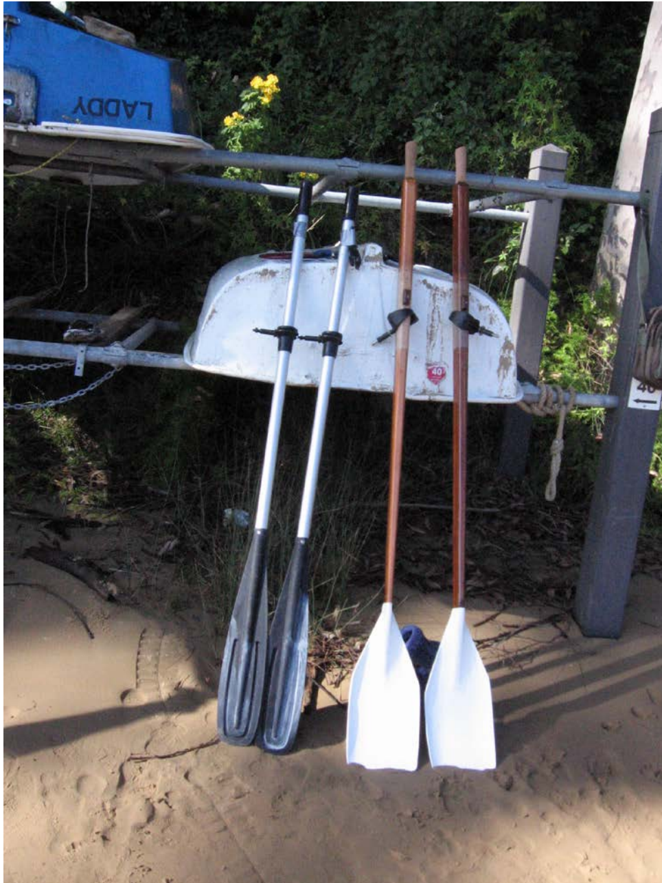
The Bic supplied oars to the left and Turbo oars with Gaco rowlocks to the right.
